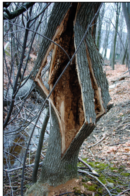
Brazier, or “hose pipe,” buckling of a white ash ( Fraxinus americana ) in a forest. The tree had a t/R ratio of about 0.1.
